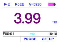
**Scan Mode**. Besides the last test thickness value, it also shows the minimum thickness value and the maximum thickness during the test.
