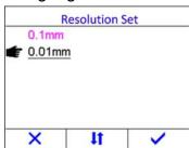
When the resolution is set to 0.01mm, the tested piece surface should be smooth to get accurate test result. When measuring rough surface or coarse grained materials, it is suggested to use low resolution.
