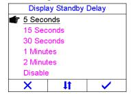
The main unit goes into standby state after a period of time as selected. Carry out a test or press any key to reactivate the main unit from standby state.
