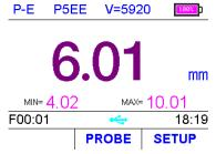
**Diff Mode**. Shows both the last test thickness value and the differential thickness value (between the absolute thickness value and the nominal thickness value)
