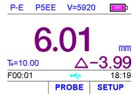
While the gauge excels at making single point measurements, it is sometimes desirable to examine a larger region, searching for the thinnest point. The gauge includes a feature, called Scan Mode, which allows it to do just that.
